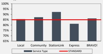
Miles between road calls (MBRC) is a vehicle reliability performance indicator that measures the vehicle miles traveled between mechanical failures for a vehicle in revenue service. Valid mechanical road calls may cause a delay in service and result in removing the vehicle from service until repairs are made. The standard for DOFR service is 14,000 MBRC and for CFR service, it is 12,000 MBRC
